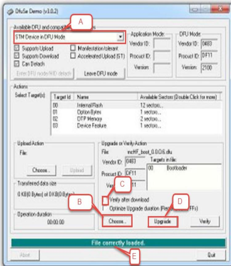
1. If you can see (A) „STM Device in DFU Mode“ in the left upper box connection between STM MCU and program is working.
