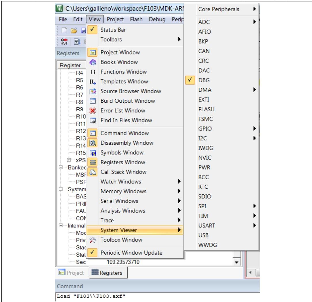
Figure 62. Accessing DBGMCU register in Keil® MDK-ARM μVision (2/2)
