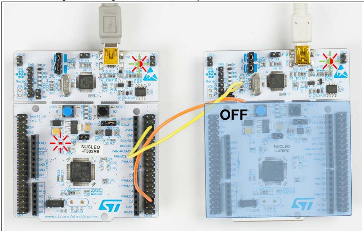
With this setup, on the PC side, two Virtual-COM ports are available with potentially two different serial channels:
