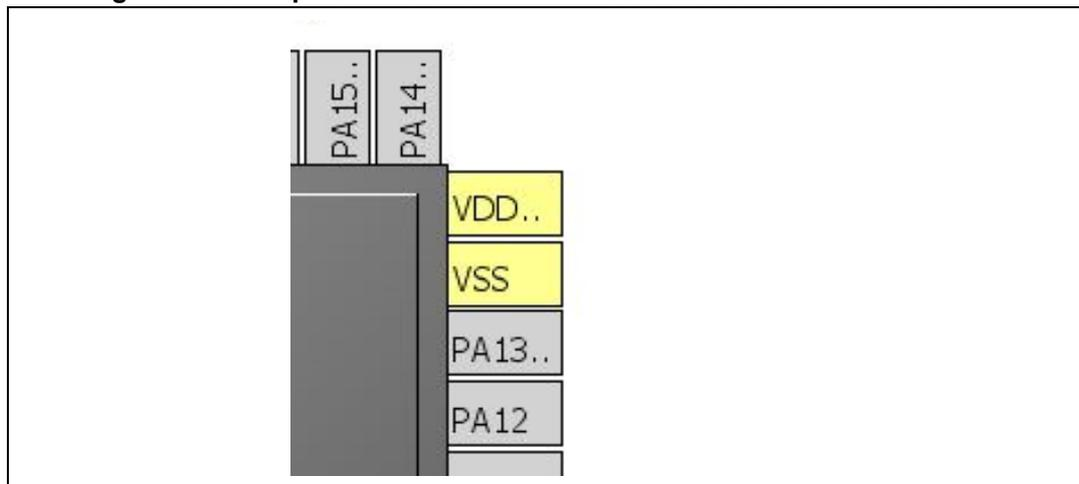
Figure 17. SWD pins PA13 and PA14 in Reserved but inactive state under STM32CubeMX
