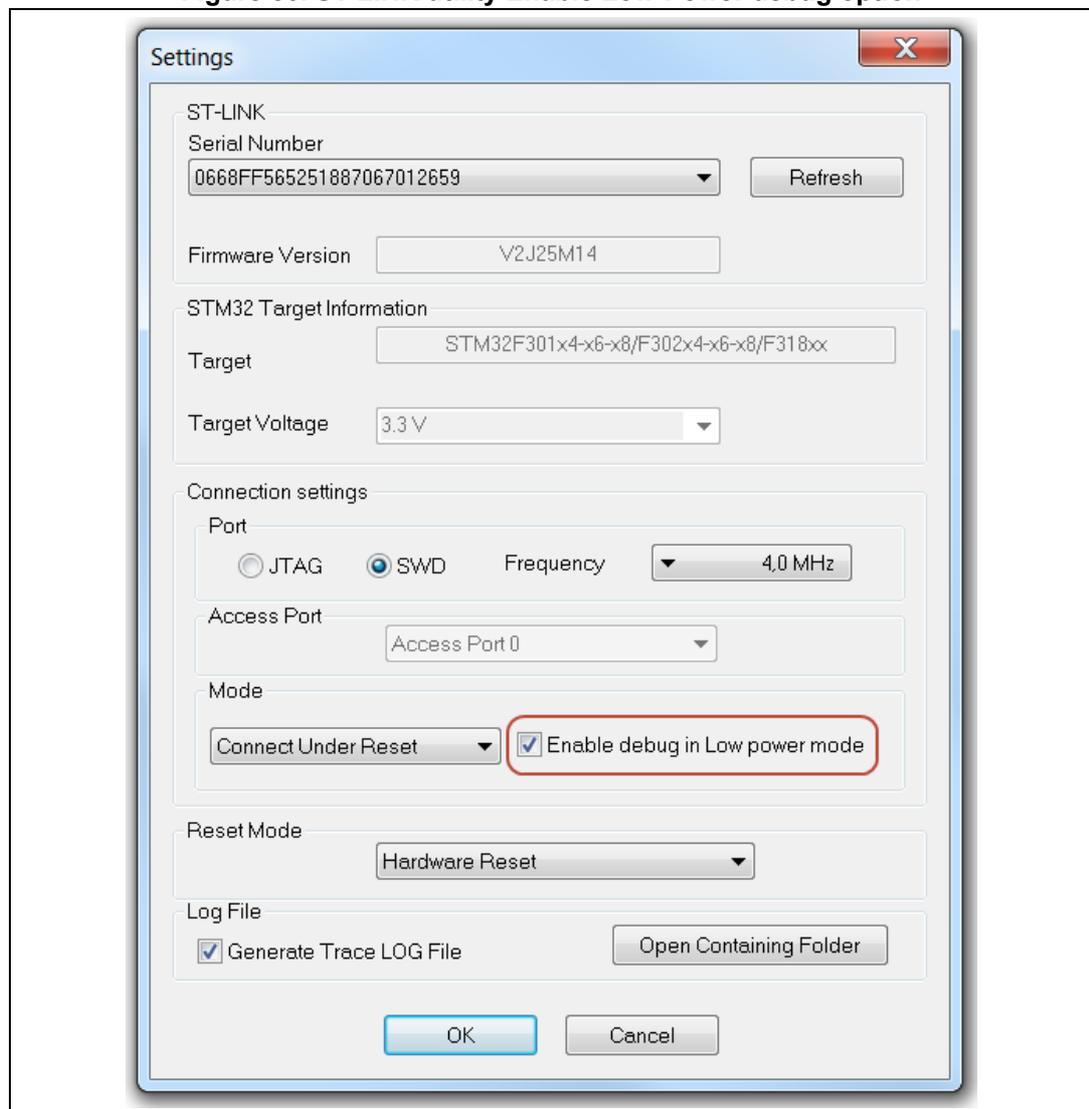
ST-LINK provides a tick box allowing to set all the three bits of DBGMCU\_CR register at once: DBG\_STANDBY, DBG\_STOP, and DBG\_SLEEP
