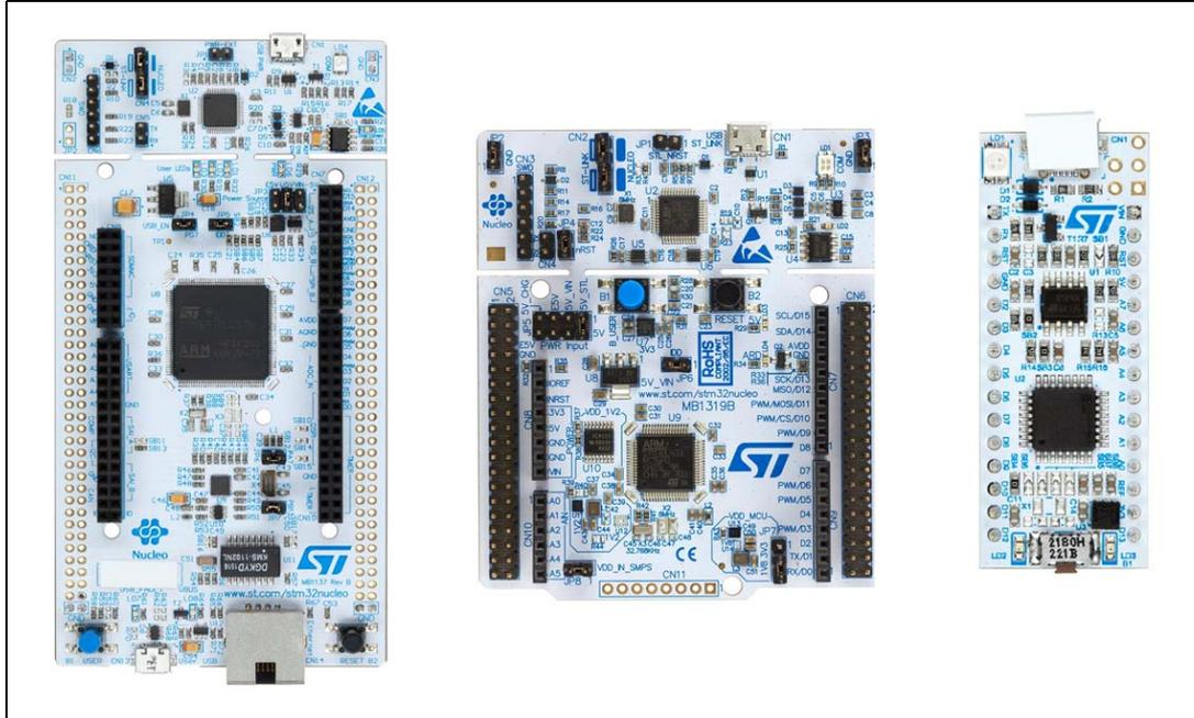
STM32 Nucleo boards feature the same connectors. They can easily be extended with a large number of specialized application hardware add-ons.
