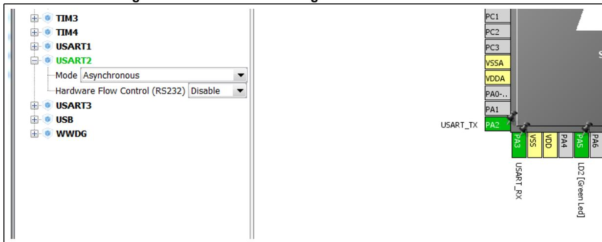
Then, set the UART communication settings in **Configuration -> USART2 Configuration -> Parameter Settings** as shown in [Figure 41](#).
