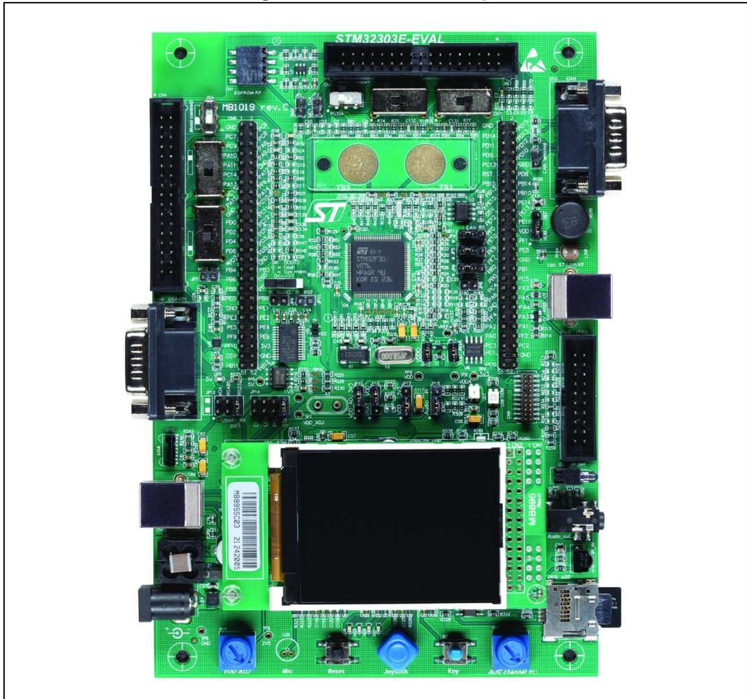
They carry external circuitry, such as transceivers, sensors, memory interfaces, displays and many more. The EVAL boards can be considered as a reference design for application development.
