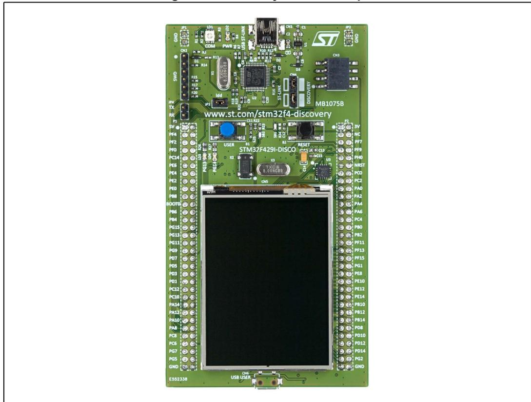
Extension connectors give access to most of the device's I/Os and make the connection of add-on hardware possible.
