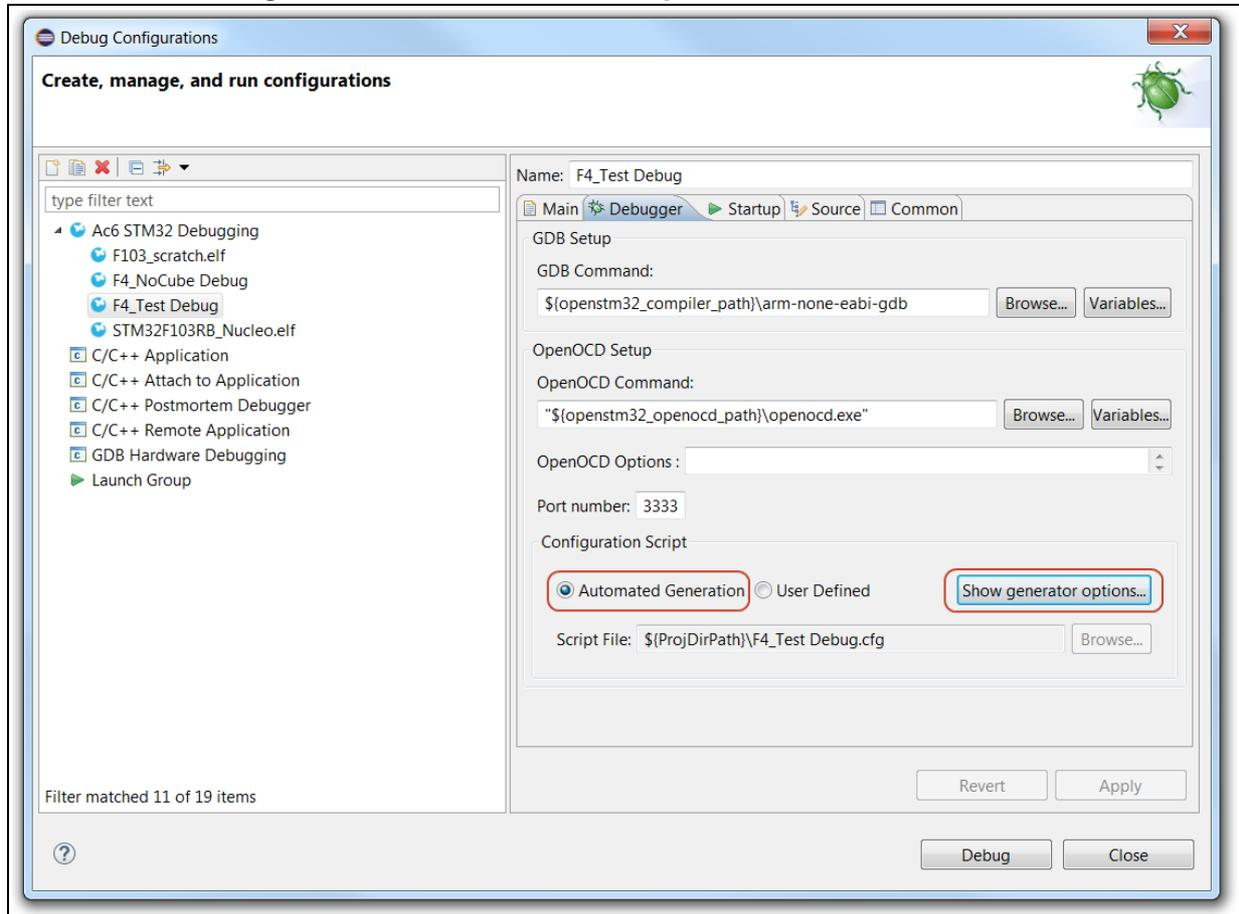
Figure 25. Select Generator Options Reset Mode in SW4STM32 V2.0.0
