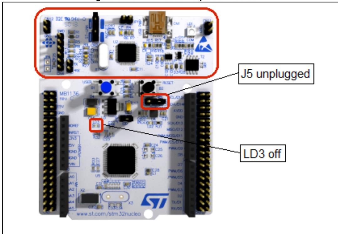
In this case the ST-LINK part can be used as a stand-alone module.
