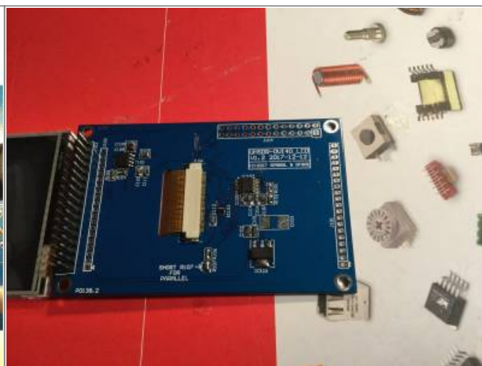
OVI40 3.5,, display, component side (photo:DL8EBD)
