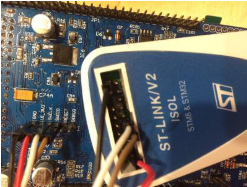
Connection ST-Link to UI board (photo F4HTX)
