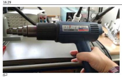
Hot air pistol used for de-soldering - see text
