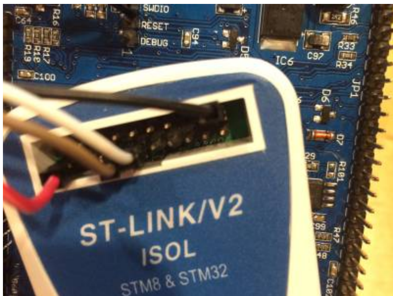
Connection ST-Link to UI board (photo F4HTX)
