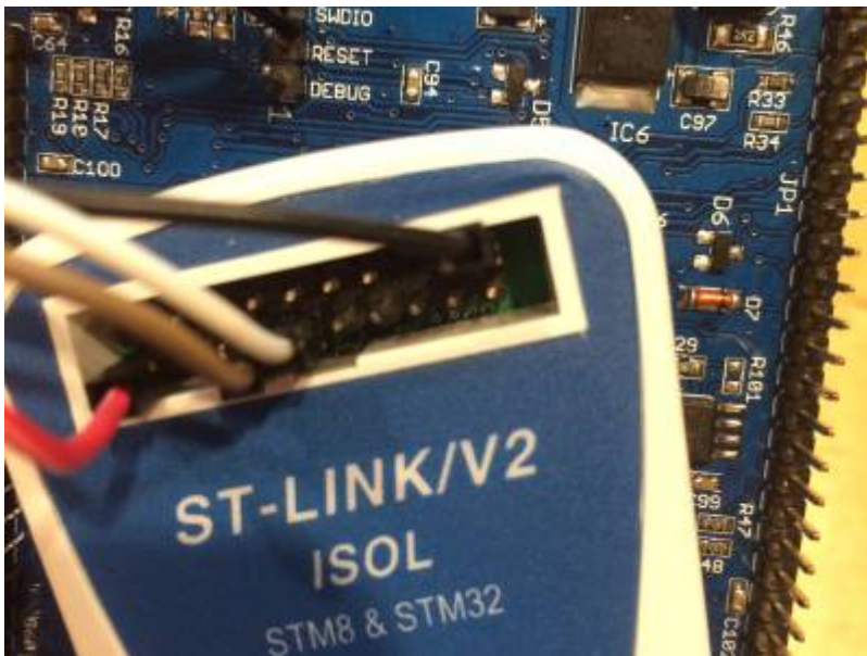
Connection ST-Link to UI board (photo F4HTX)
