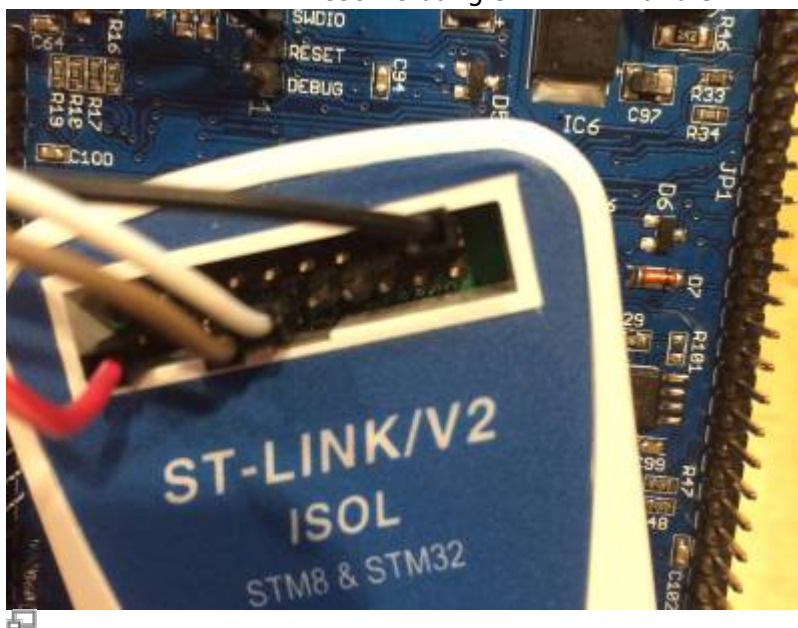
Connection ST-Link to UI board (photo F4HTX)
