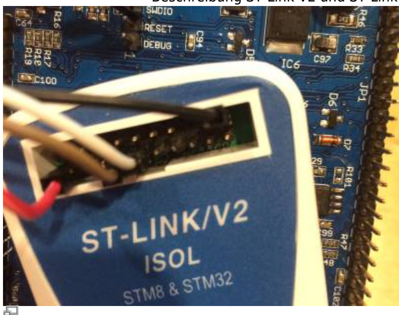
Connection ST-Link to UI board (photo F4HTX)
