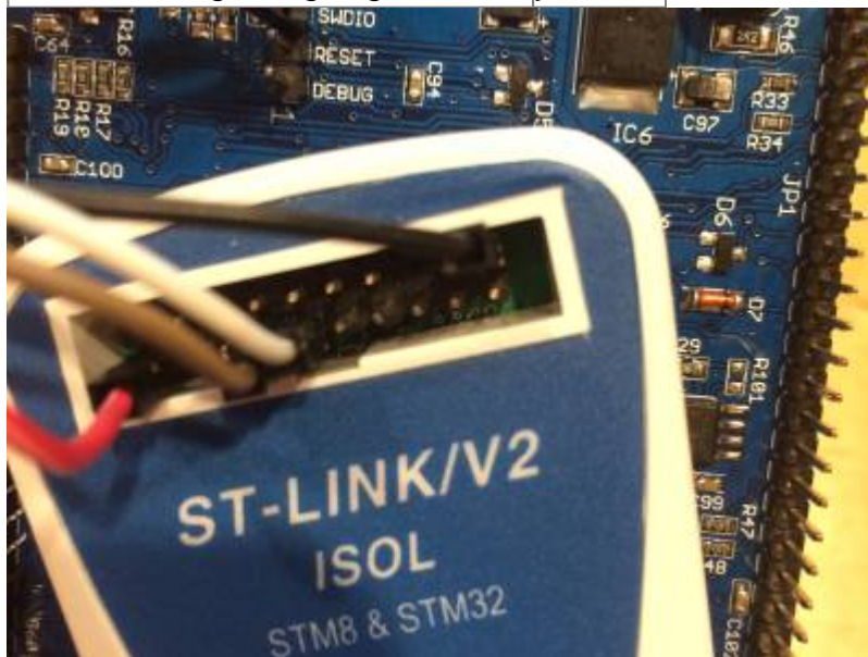
Connection ST-Link to UI board (photo F4HTX)
