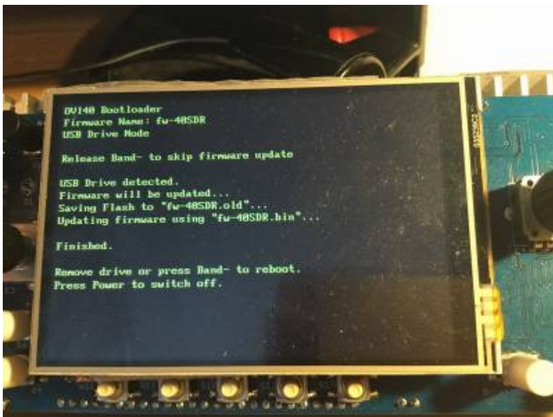
Bootloader Upgrade per USB Stick (Photo DL8EBD)
