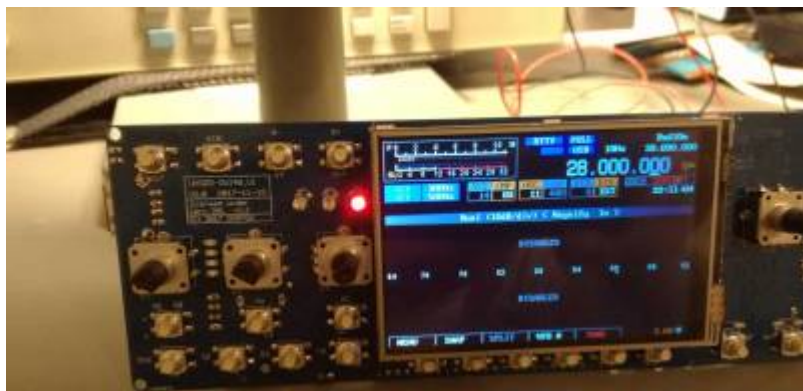
OVI40 UI and display board (photo DF9EH)
