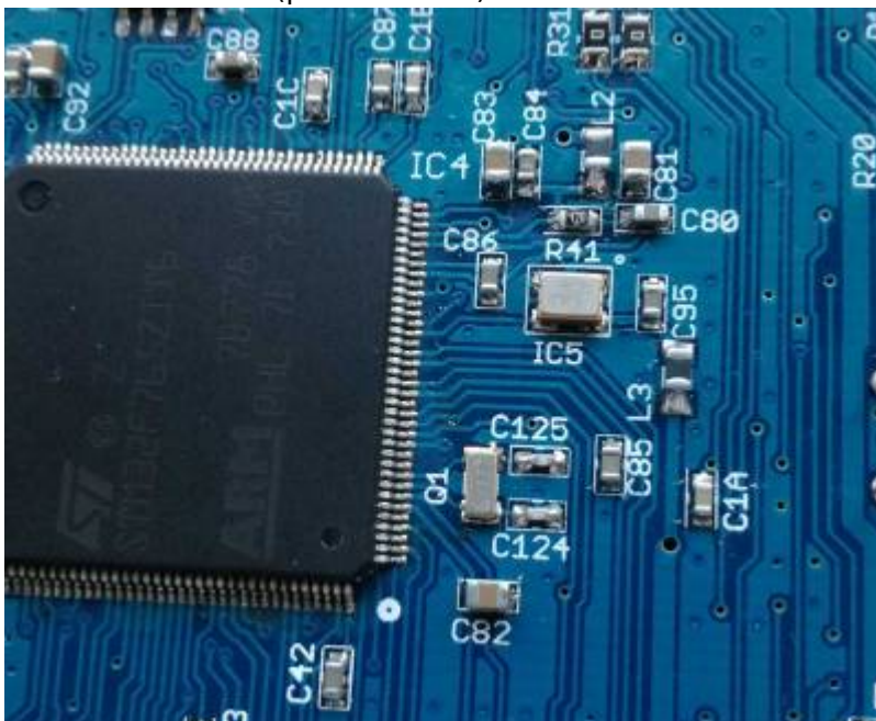
Orientation of TXCO & MCU (photo DF9EH)
