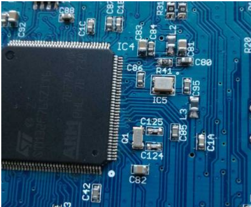
Orientation of TXCO & MCU (photo DF9EH)
