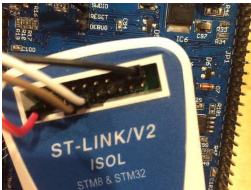
ST-Link connection to UI board (Photo F4HTX)
