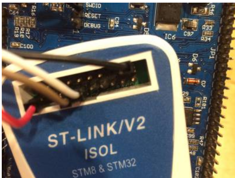
ST-Link connection to UI board (Photo F4HTX)
