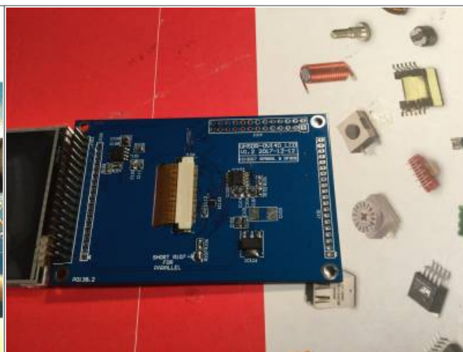
OVI40 3.5,, display, component side (photo:DL8EBD)
