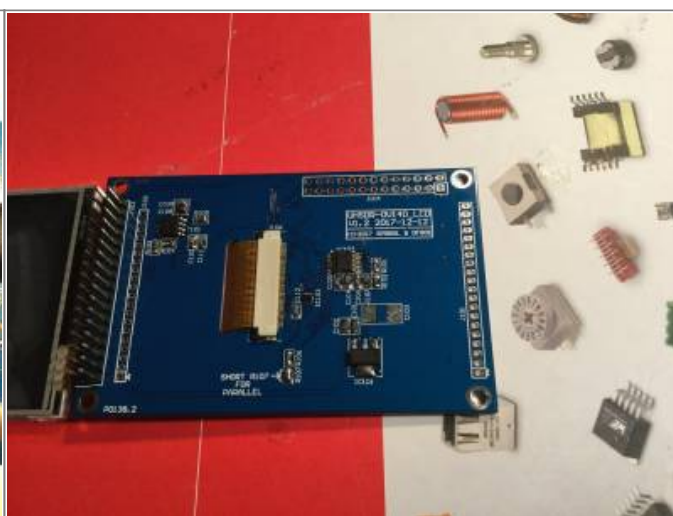
OVI40 3.5,, display, component side (photo:DL8EBD)
