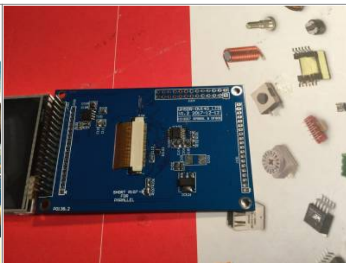
OVI40 3.5,, display, component side (photo:DL8EBD)
