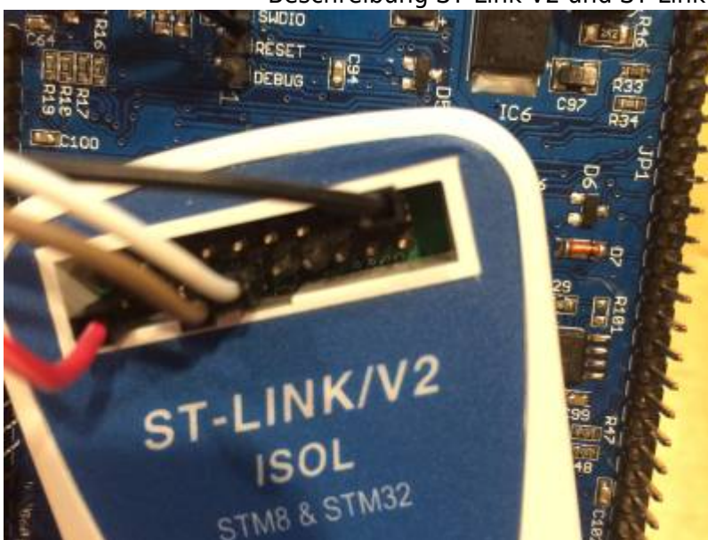
Connection ST-Link to UI board (photo F4HTX)
