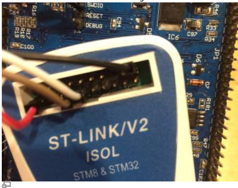
Connection ST-Link to UI board (photo F4HTX)
