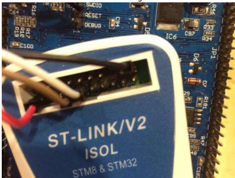
Connection ST-Link to UI board (photo F4HTX)
