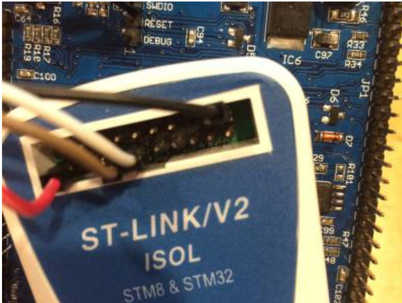
Connection ST-Link to UI board (photo F4HTX)
