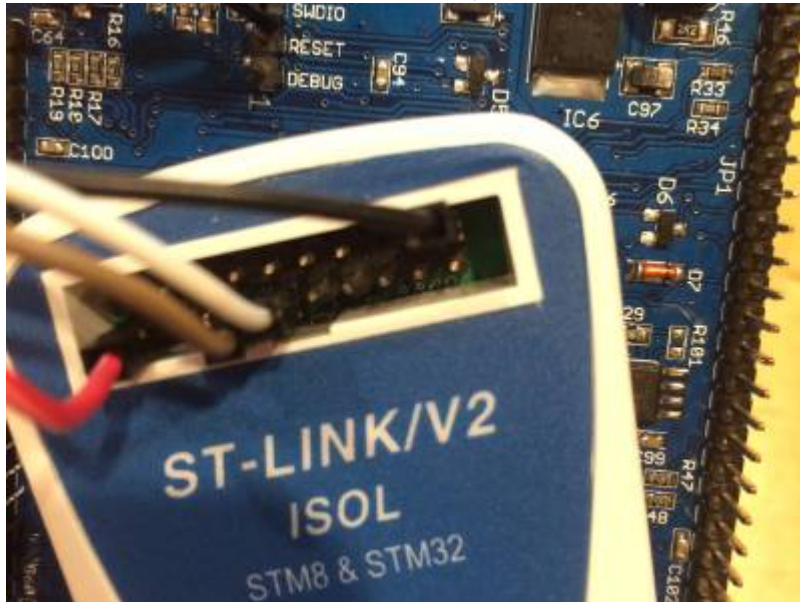
Connection ST-Link to UI board (photo F4HTX)
