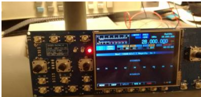
OVI40 UI and display board (photo DF9EH)
