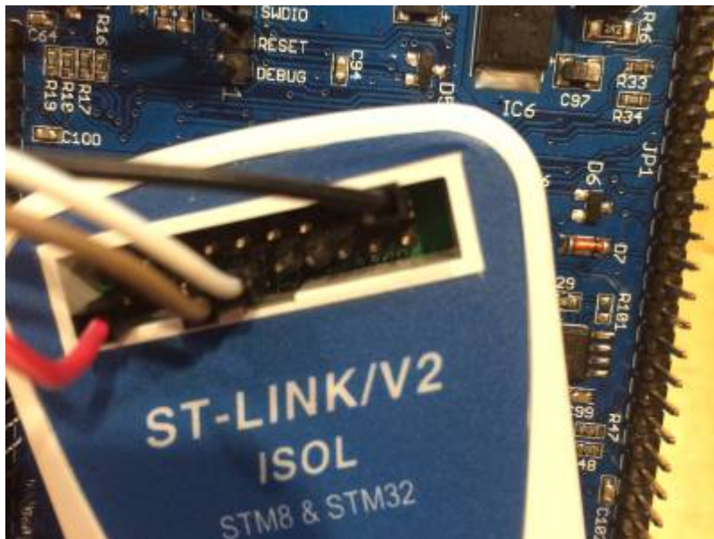
Connection ST-Link to UI board (photo F4HTX)
