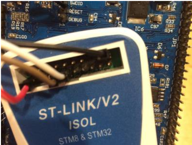
Connection ST-Link to UI board (photo F4HTX)
