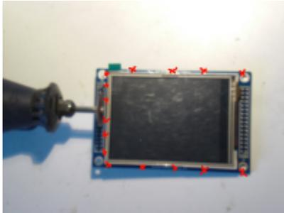
panel where the flat ribbon cable runs out need to mandatory kept ! On the left side where the soldering holes were cut off we have the potential danger that copper strips from the pcb were shortened by the metal frame of the panel. This can easily be avoided with a small piece of scotch tape. Lift the panel ca. 0.5mm very carefully with a cutter knife and place the scotch tape under it. Fold it over the pcb edge. If you do not have an LCD with double lines connector strips at the right
