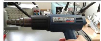
Hot air pistol used for de-soldering - see text
