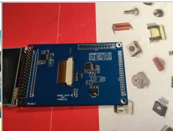
OVI40 3.5,, display, component side (photo:DL8EBD)
