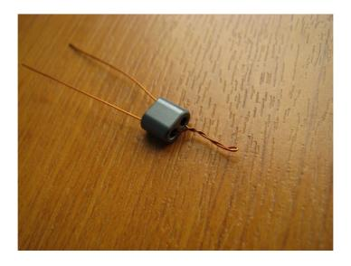
Then route the first end into the opposite hole to form the first turn of the secondary:
