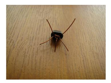
Finally the transformer is complete, please carefully scrape the ends with a sharp SMD tool, then using plenty of flux (resin) and solder, prepare them and insert.
