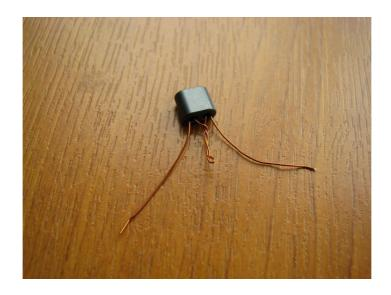
Now using the rest of the wire, we do the primary, so we form the first turn, where one turn in a binocular core is when a wire goes through both holes and exits on the same side it enters:
