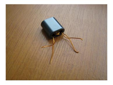
Finally scrape the ends, and prepare them with flux and solder, then insert:
