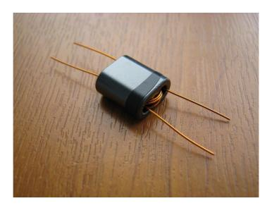
Finally, scrape the ends, cover with flux and solder and push through:
