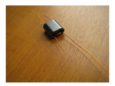
Complete the full 3 turns and mark this side with some tape, for easier identification later:
