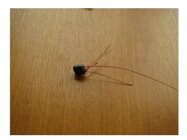
Continue with the rest of the turns, until we have full 4 turns. Be careful while pushing the wires, as it is tight fit, do not scrape the coating, as this could short the transformer:
