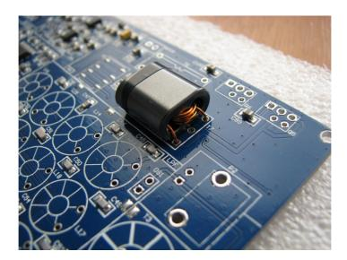
Please make sure you insert the correct way – primary 2 turns goes to the transistors (pointing the P2 connector footprint).
