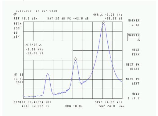
Right peak: main side band, center peak: poorly suppressed carrier, left peak opposite side band.
