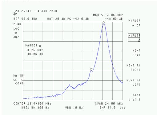
Unfortunatelly there is only last spur visible: 3kHz below the main side band (4\*750). It can be seen that 300Hz RBW of spectrum analyzer is not sufficient to see spurs. FFT of ordinary sound card with simple SDR receiver would have better frequency resolution.
